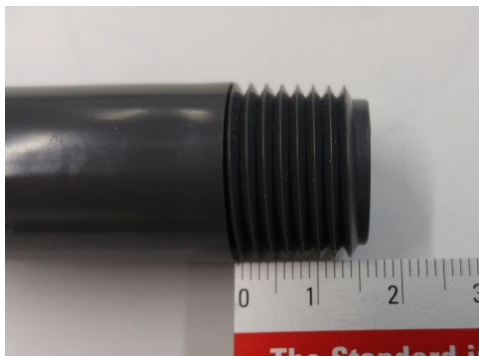
Typical 1/2" tapered thread length
