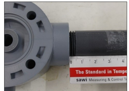
Thread depth at 1-1/2 turns.
