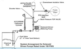
Back Pressure TOP VALVE ACCU-PULSE Downstream Isolation Valve Pressure Relief TOP VALVE PFS Injection ACCUDRAW Calibration Antor Driven oot Valve 3" - 6" from Tank Bottom) Chemical Tank System Arrangement for Solenoid Driven (Above 150 PSIG) or Motor Driven Pumps
